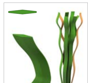
Fibre thickness: approx. 120 µm
